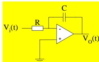
$$V_o(t) = V_o(0) - \frac{1}{RC} \int_0^t V_i(t) dt$$
